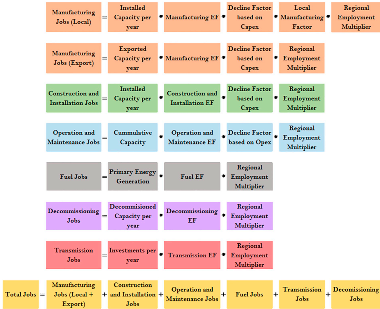
Fig. 1. Method for estimation of job creation during the energy transition. Abbreviations: Employment Factor (EF), Capital Expenditure (CAPEX) and Operational Expenditure (OPEX).
